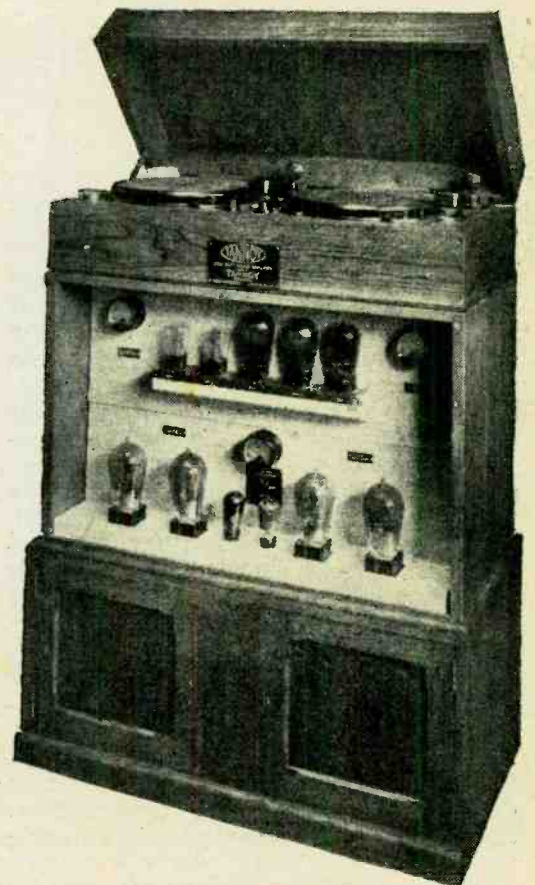
A 1-KILOWATT AMPLIFIER. The Tannoy battery-operated gramophone console and amplifying equipment installed in the "Daily Mirror" van now touring the health resorts.
