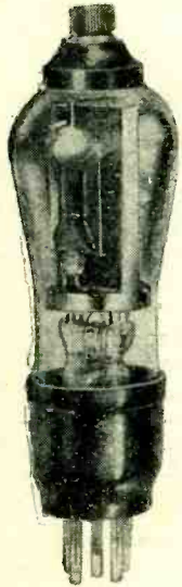
Osram VDS, an indirectly heated variable-mu valve for D.C. mains.
